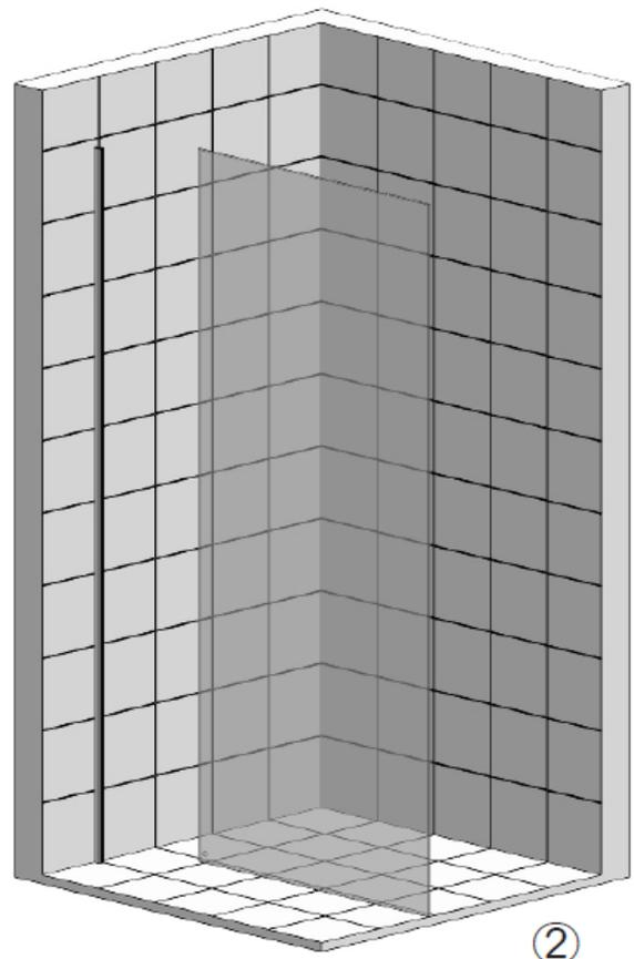
1. Place a bead of silicon vertically on the inside of the Wall Channel.
